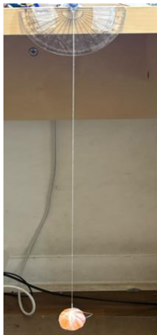
Figure 1a. A bouncy ball of mass 14.141 g hangs by a 0.4000 m string over a pencil that extends 3.00 cm off the edge of a table. A protractor is taped behind the pendulum to measure angular displacement.
